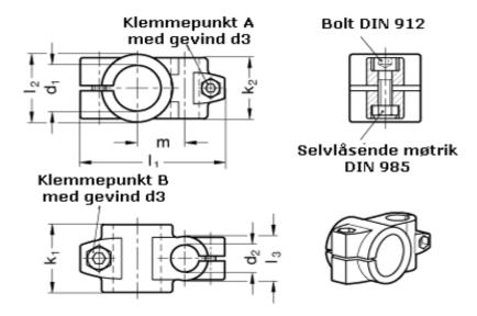
Adjustable clamp lever for d3 = GN 911-M 8-32 have to be ordred separately Adjustable clamp lever for d4 = GN 911-M 6-25 have to be ordred separately d1 = 25 d2 = 12 d3 = M 8
